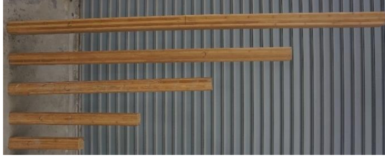
Fig. 22 LBL columns with different slenderness ratios
