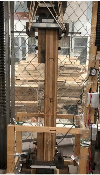
Fig. 5 (a) Eccentric compression test
