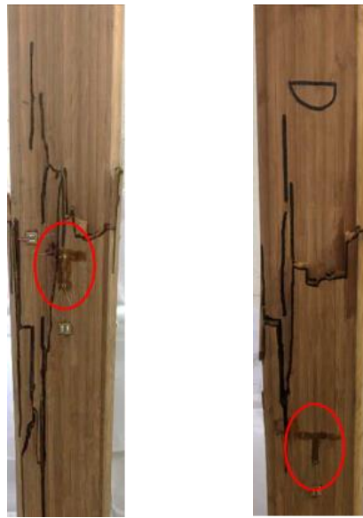
Fig .8 Cracking position (a) near the center (b) far from center
