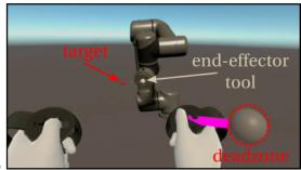
Figure 4.3: The experimental task and experimental setup: a) illustration of the experimental task - the operator needs to bring the end-effector tool to the target using rate mode; b) operator uses Oculus Quest 2 headset and Oculus Touch controllers to teleoperate the robot in VR; c) operator's VR view (similar to illustration in a)).
