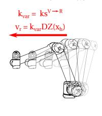
Figure 4.2: Constant and variable rate mode control. For the same displacement of the input device following rate modes can be used: a) constant rate mode, that does not change with the virtual world scale; b) variable rate mode, that changes along with the virtual world scale
