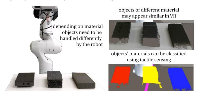
Figure 3.5: Object material visualisation in VR: objects of different material appear similar when rendered as point clouds in VR, which in turn can lead to operator taking incorrect decisions. Tactile sensing can be used to classify objects' materials and communicate them visually to the operator.
