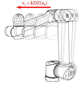
b) variable rate scaling dependant on the virtual world scale, for example: virtual world scaled to a half of real  $s^{V \rightarrow R} = 0.5$
