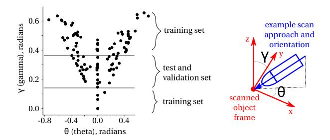
Figure 3.7: Distribution of different initial tactile scanning angular orientations of the sensor.  $\gamma$  is the angle between the objects' surface normal and the tactile sensor's z axis.  $\theta$  is the angle between the projection of the tactile sensor's z-axis to the scanned object's xy-plane and the object's x-axis (object's x and y-axis are collinear with the robot's with an origin and desired scan position).
