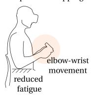
Figure 4.1: Input device workspace comparison in position-position and position-rate mapping modes. Smaller arm movements can be used in rate mode, leading to reduced fatigue: a) the operator is using full arm movements in position-position mapping to control the robot; b) the operator is using elbow-wrist movements, while arm is constrained to control the robot in rate mode.
