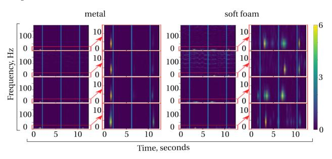
Figure 3.11: Sample spectrograms (not normalised) for metal and soft foam. There are large spikes in 0-15Hz frequency range for both materials (arrows indicate zoom-in regions) and smaller spikes in high frequency for softer/rougher soft foam.
