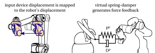
Figure 2.6: Direct position-position control mode. Change of pose of the leader device is mapped directly to change of pose of the follower robot. Top: unilateral direct position-position mode control using VR handheld controllers; bottom: bilateral direct position-position mode control using haptic device.
