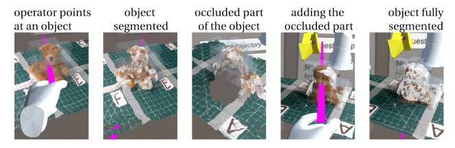
Figure 2.4: Object segmentation illustration
