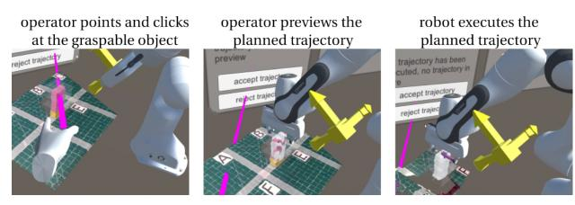
Figure 2.9: Supervised control mode: point-and-click grasping
