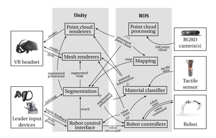
Figure 2.1: VR-based robot teleoperation framework scheme
