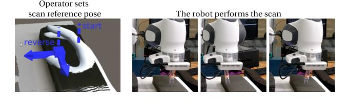
Figure 2.10: Supervised control mode: tactile scanning
