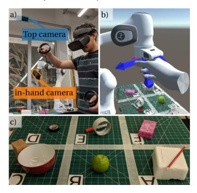
Figure 3.1: VR-based robot teleoperation with end-effector mounted camera
