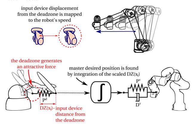
Figure 2.7: Direct position-rate control mode. Displacement from the deadzone of the leader device is mapped to the rate of the follower robot. Top: unilateral direct rate control using VR handheld controllers; bottom: bilateral direct rate control using haptic device.
