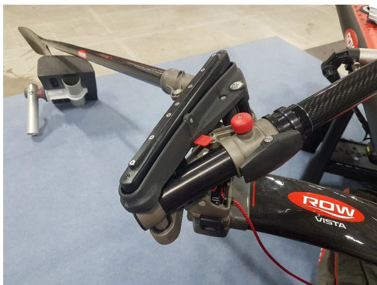
Row Vista mechanism for reversing oar motion
