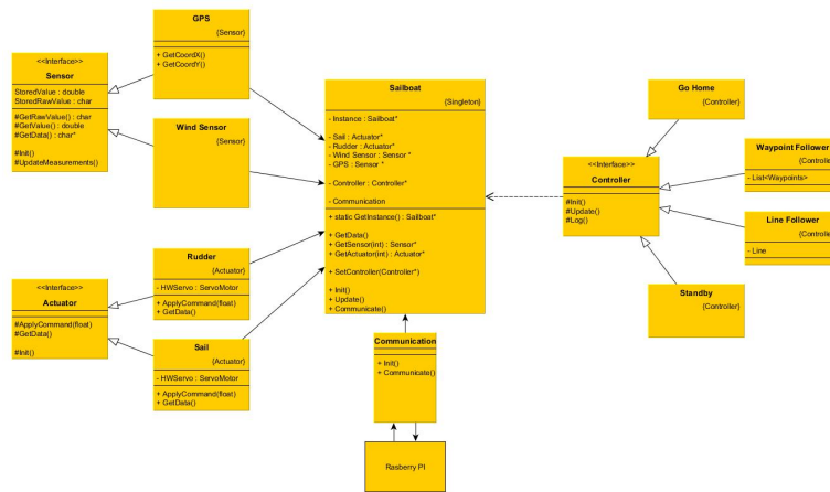
Figure 3: UML of the Component-Based Architecture.
