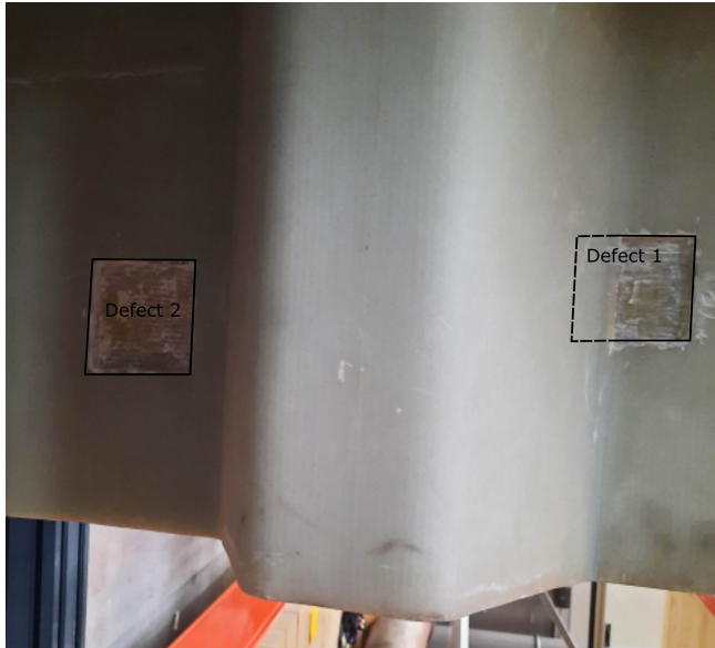
FIGURE 6: Artificial defects embedded within the surface. Their dimensions are 10\text{cm} \times 10\text{cm} since defects below this threshold are not considered critical. Defect one represents a delamination of the stiffener member, cutting through the stiffener and intersecting the non-structural core with a depth of 0.2\text{cm} from the outside of the hull. A portion of the defect is present under the structural foam, represented by the dotted line. Defect two represents internal tear and wear to the hull's skin with a depth of 0.5\text{cm} from the outside of the hull. The image is reflected and rotated anti-clockwise by 90^\circ relative to the images produced as a result of scanning later.
