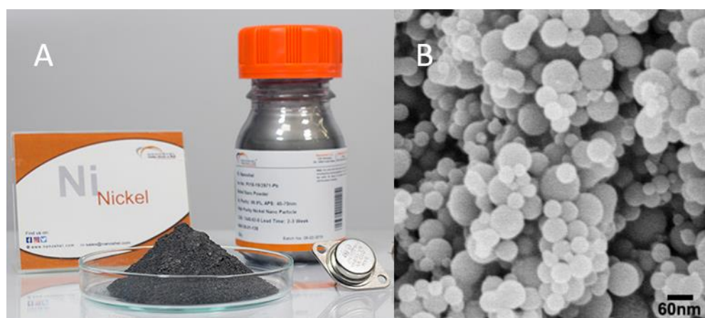
Figure 1.2 A – Nickel nanoparticles (NiNPs), or nickel nanopowder. B – NiNPs seen through electron microscopy (scale bar = 60 \mu m). Source: A – www.nanoshel.com ; B – www.ssnano.com .
