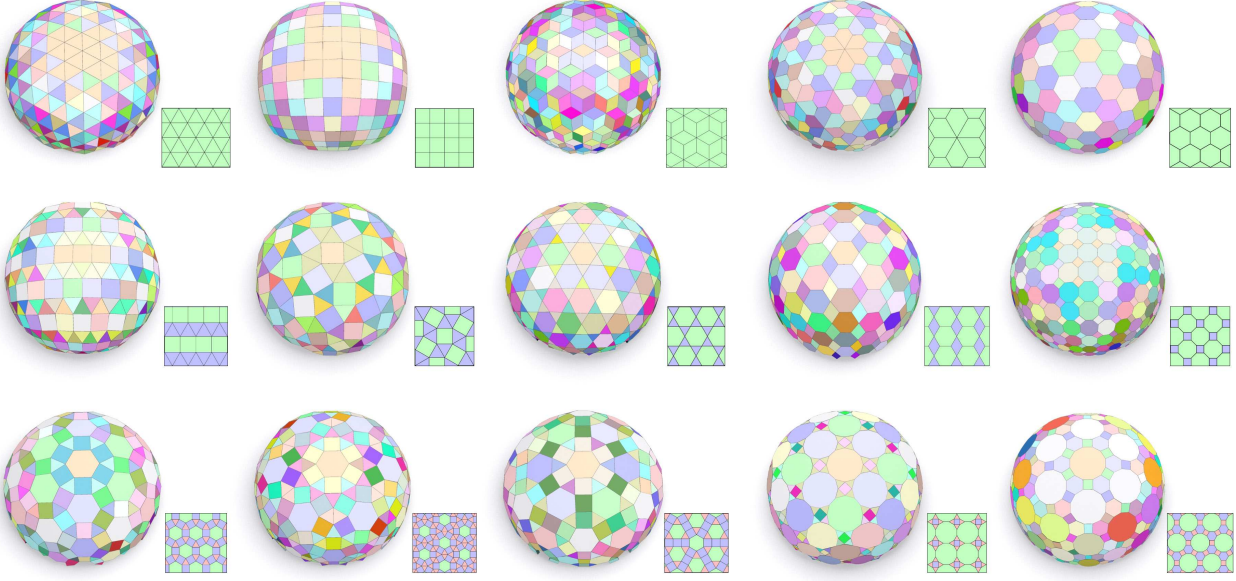
Fig. 12. Our approach allows generating results with a variety of patterns of a DOME surface, where the corresponding 2D tessellation is shown in the boxed image. The 2D tessellations in the top, middle, and bottom rows are monohedral, dihedral, trihedral tilings, respectively. For each result, shell elements falling in the same discrete equivalence class are rendered with the same color.
