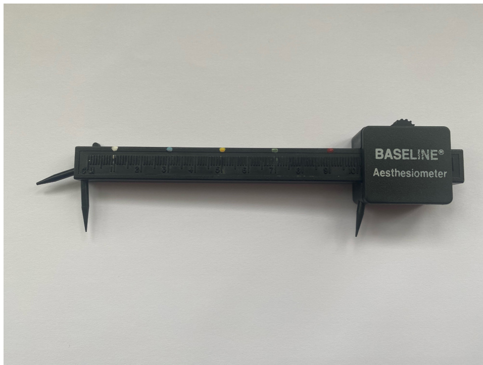
Figure 4 The marked two-point discrimination tool.
