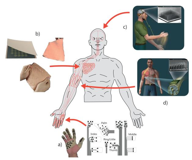
Figure 3: **Representative examples of interfaces that can provide high-bandwidth tactile stimulation**: a) High-density matrix electrodes for electrotactile stimulation (30), b) Skin-integrated multichannel vibrotactile interface (32), c) Utah electrode arrays for brain stimulation (33), and d) Utah slanted electrode arrays for peripheral nerve stimulation (33).
