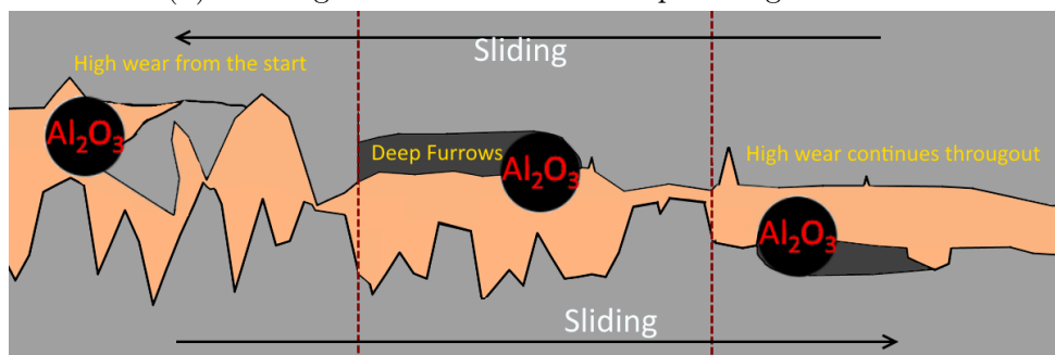
(c) Film thickness smaller than diameter of particle, \text{Al}_2\text{O}_3 causes massive wear.
