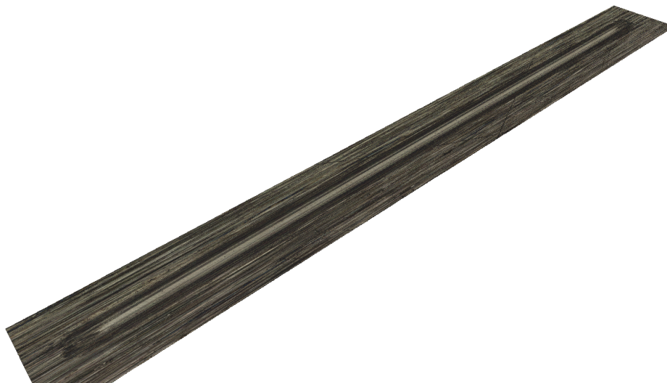
Figure 6.11: A true colour 3D image of the Lith-Moly wear scar taken in the Alicona.
