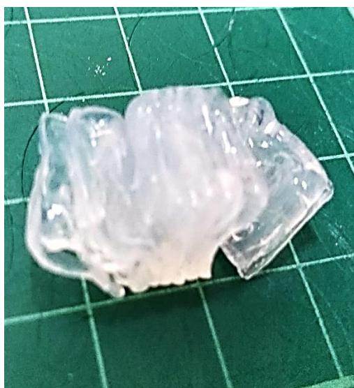
Figure 3.7: A printed 12 mm \kappa C-thiamine hydrogel cube that has delaminated after undergoing compression testing. Each square on the grid shown is 10 mm 2
