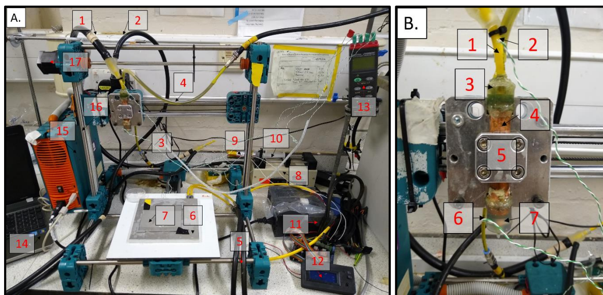
Figure 4.1: Schematic of the retrofitted Fabbster printer (A) including 1) Jacketed pipe from the syringe to the nozzle, 2) Jacketed pipe from the nozzle to the water bath, 3) Jacketed pipe from a water bath to the bottom of the nozzle, 4) Pipe from the top of the nozzle to the water bath, 5) Jacketed pipes to and from a water bath to the temperature controlled bed, 6) Temperature controlled printing bed 7) Removable section of the printing bed 8) Syringe driver, 9) Heating jacket, 10) 60 mL syringe, 11) Power supply unit, 12) Controller for heating jacket, 13) Data logger, 14) Laptop to control printer, 15) Controller unit for the printer, 16) Support rods for the printer, 17) Support rods and motor for the printer. (B) Schematic of the printer nozzle including 1) Feed pipe into the nozzle, 2) Thermocouple to monitor temperature of feed material as it enters the nozzle, 3) 3D printed part to connect feed pipe to the copper pipe, 4) Copper outer pipe containing brass inner pipe, 5) Bracket to hold copper pipe in place, 6) Thermocouple to monitor temperature of feed material as it enters the die, 7) 3D Printed nozzle. The printer was connected to and controlled by a computer running Netfabb for Fabbster software.
