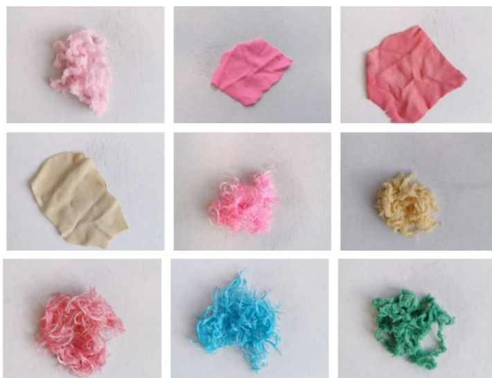
Figure 7.17: Polyester fibers and fabrics dyed with recycled synthetic dye using [DMBA][HSO 4 ] dye extraction-dyeing process
