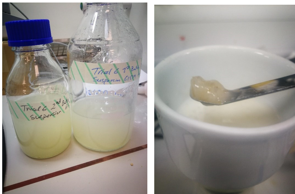
Figure A26: nanocellulose suspension after alkaline oxidation using H_2O_2 (left) suspensions right after the oxidation reaction and (right) gel-like material upon filtering the suspension
