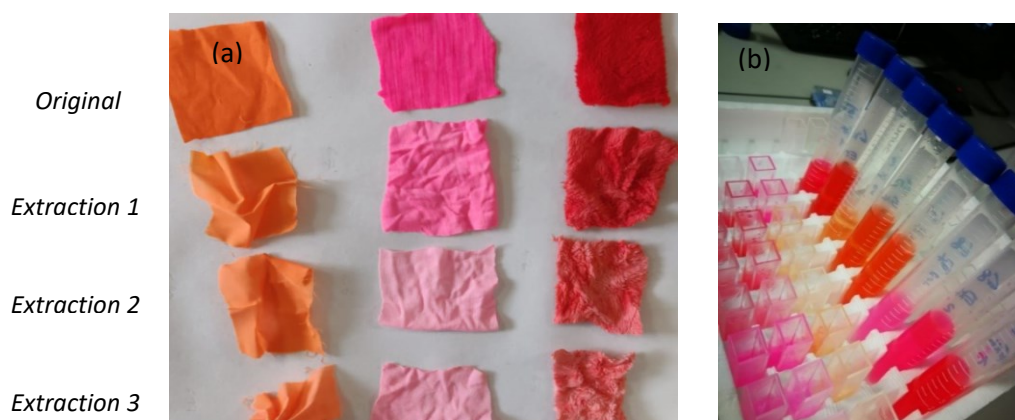
Figure 7.10: (a) Original photograph of original fabrics and the dye extracted fabrics from extraction 1 to 3 (b) ionic liquid + dye solutions after the dye extraction experiments
