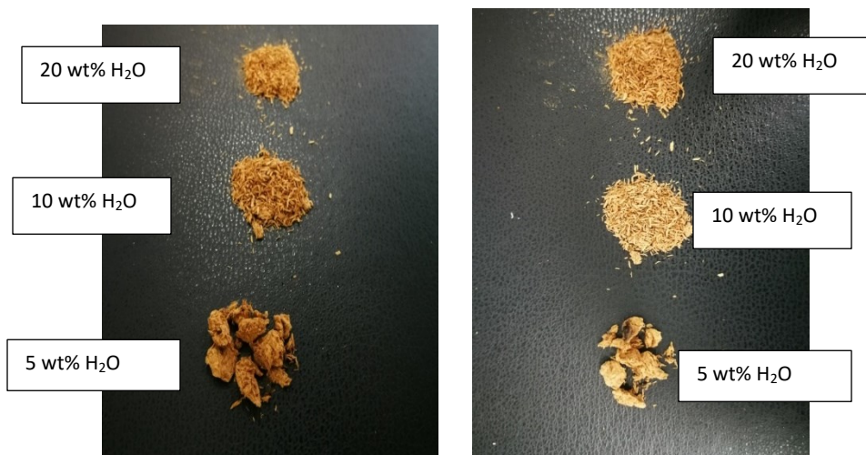
Figure A22: Cellulose pulp from pretreatment with [DMBA][HSO_4] mixed with different water concentrations. (Left) softwood pine pulps and (Right) Miscanthus cellulose pulps
