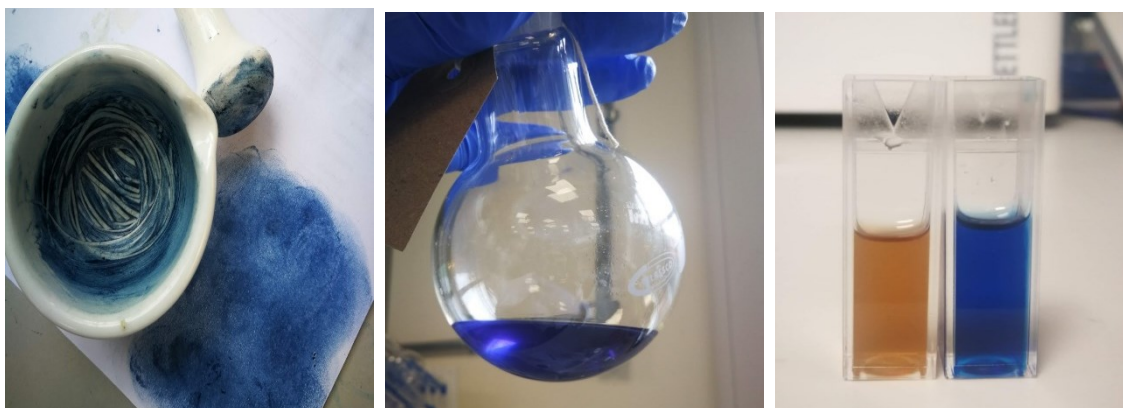
Figure 7.21: a) pigmentation effect of the generated cotton powder, b) cotton powder in DMSO solvent and, c) pale-yellow IL solution after treatment exposed to air and blue coloured IL that was kept under N_2 after the treatment
