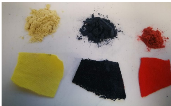
Figure 7.23: Cotton pieces before being treated with 80 wt% [DMBA][HSO 4 ] (bottom) dyestuff pigments made of cotton after treatment with 80 wt% [DMBA][HSO 4 ] (top)
