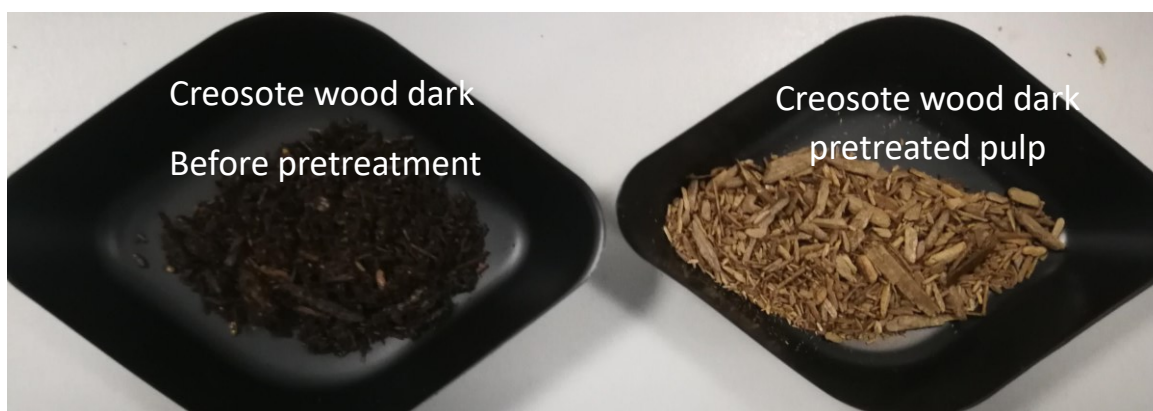
Figure A19: Creosote wood dark before pretreatment and creosote dark pulp after pretreatment using [DMBA][HSO_4] at 170 °C and 45 minutes
