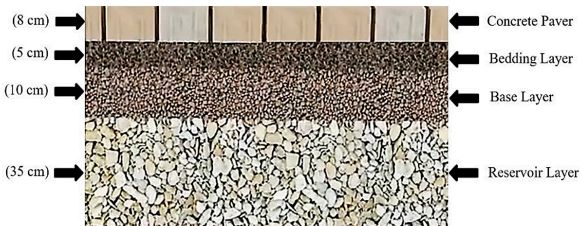
Figure 14. Layer thicknesses of PICP.
