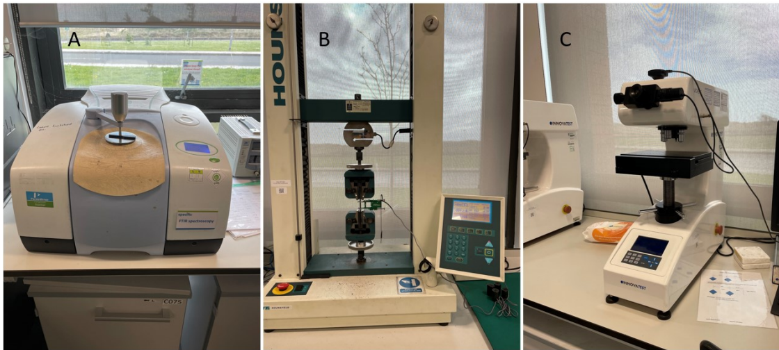
Figure 4.3 - Testing apparatus A) Perkin Elmer Frontier FT-IR spectrometer. B) Hounsfield H25KS. C) Innova Test Vickers hardness testing rig
