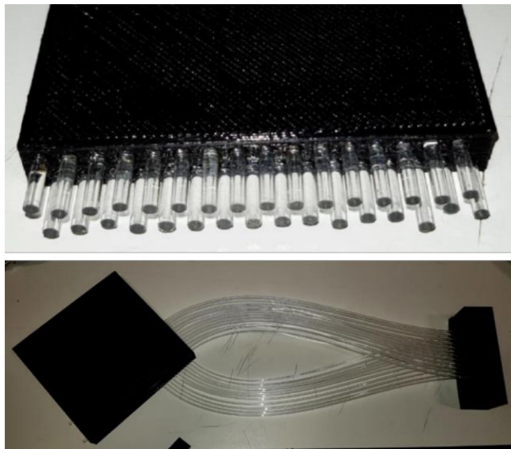
Figure 1.4 – 3D printed muon detector structure by 3D Scint. 32 x 2mm fibres on each axis, giving 64 channels.
