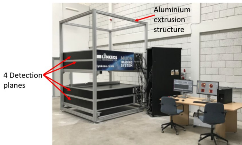
Figure 1.3 – Lynkeos muon imaging system (MIS) fully assembled at The University of Glasgow
