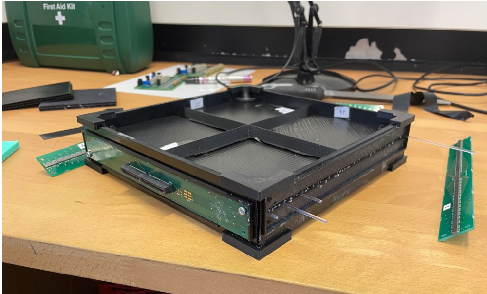
Figure 3.10 – Complete assembly of the novel design proposal. Inc. 3D printed components, Fibres, and SiPMs
