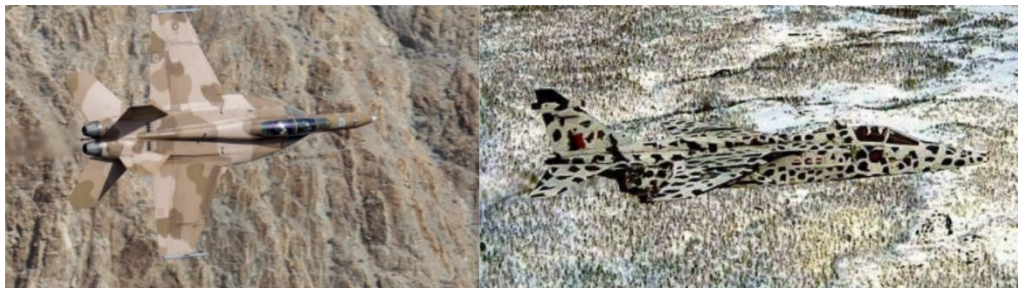
Figure 2-17 - Visual signature reduction through camouflage paint
