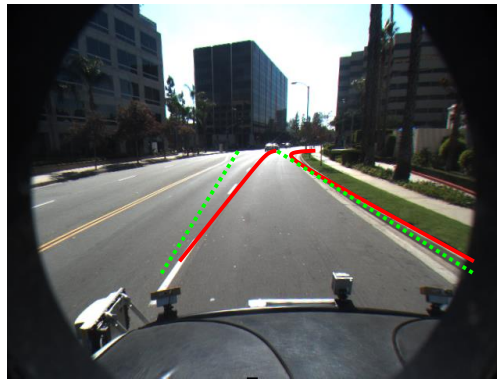
Figure 4-9. Compensation of the secondary lane detection algorithm.
