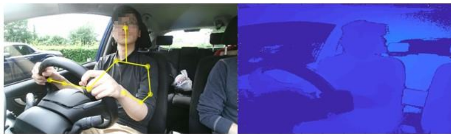
Figure 5-2. Driver body joints detection with Kinect.
