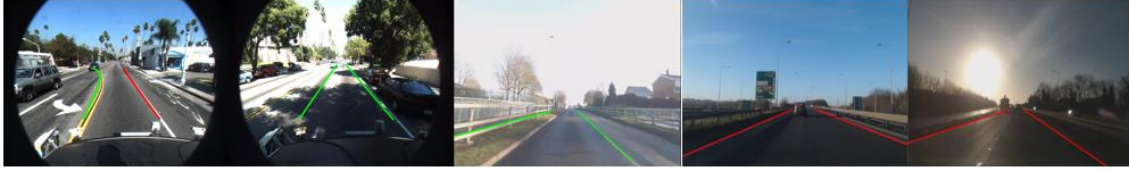
Figure 4-11. Inaccurate and false detection samples showing the influence of curbs, no or poor lane marks, lane changing and model weakness.
