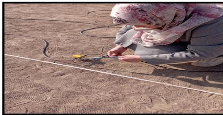
Fig. 3. The process of connecting the geophone (S) to the cable to convert the signal into a seismograph
