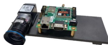
Figure 6 3D Printed design platform and fixed sensors
