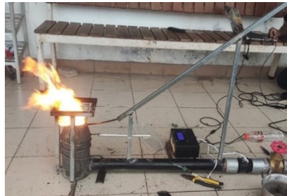
Fig. 16. The flame is at an air pressure of 7.11 Pa
