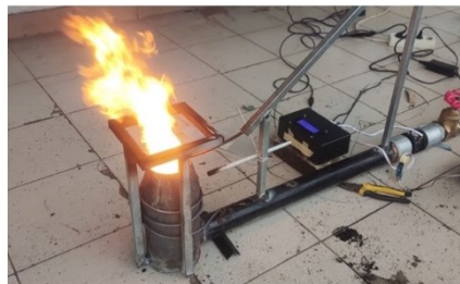
Fig. 14 The flame is at an air pressure of 3.004 Pa
