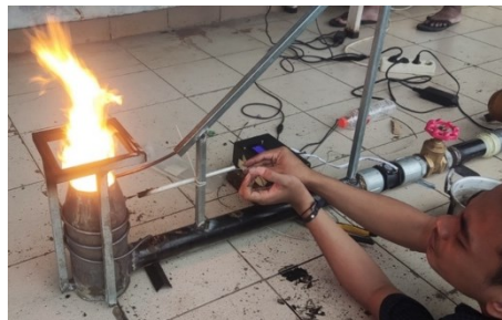
Fig. 20. The flame at air pressure 18.78 Pa
