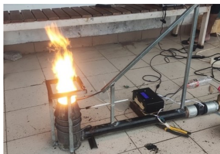
Fig. 22. The flame at air pressure 27.04 Pa
