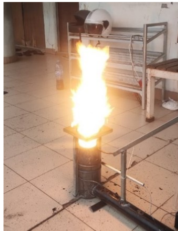
Fig. 24. The flame at air pressure 39.06 Pa
