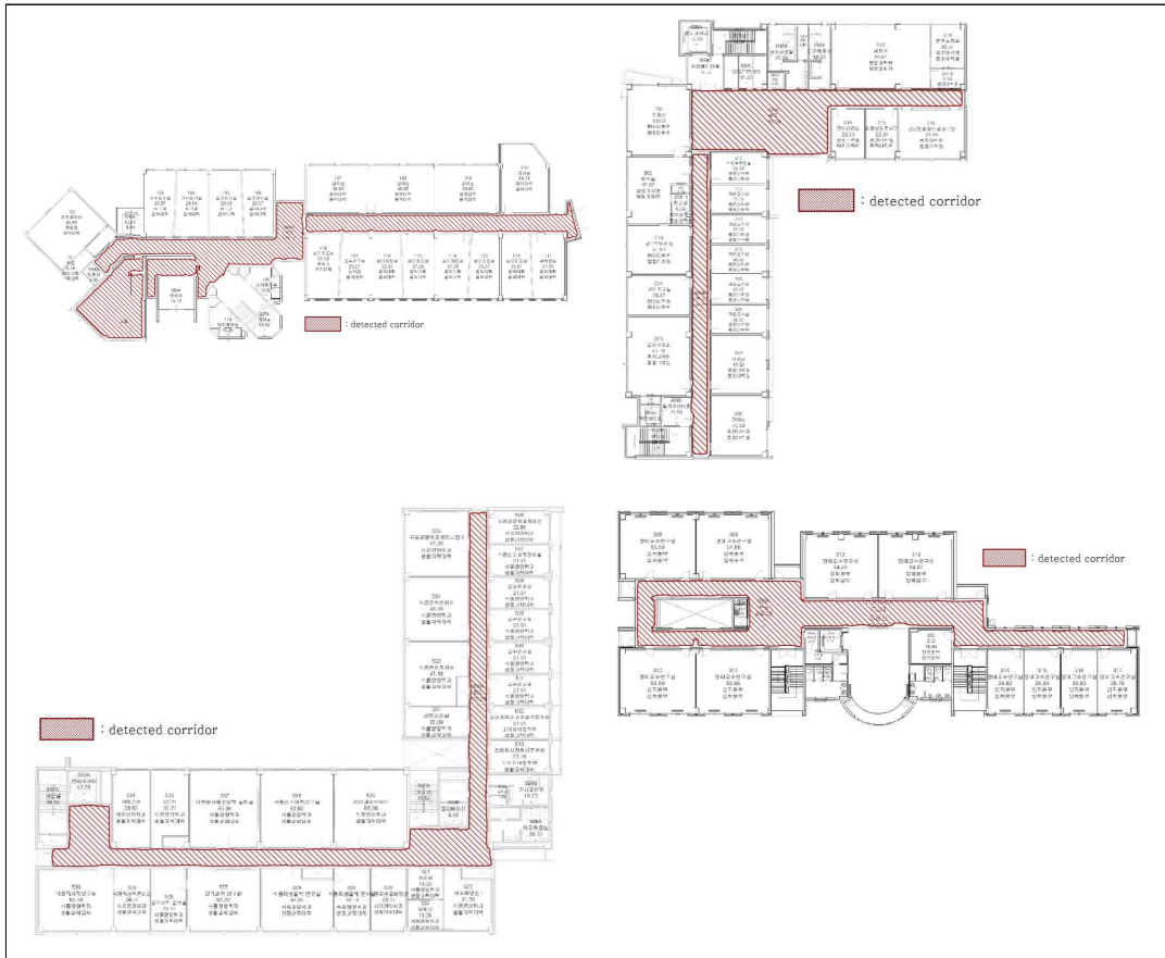
[Figure 4-3] Detected corridors of test floor plans C, D, F, and G (in clockwise order from top left)
