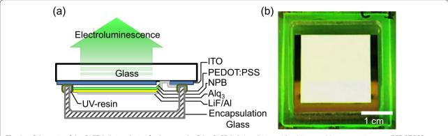
Fig. 8 a Schematic of the OLED lighting device, **b** photograph of the OLED lighting device with a 20 mm × 20 mm emission area (PEDOT:PSS deposited by micro multi-nozzle jet coating)
