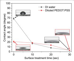
**Fig. 5** Variation of contact angles of D.I. water and diluted PEDOT:PSS liquids on the ITO-deposited substrate with the  $\rm O_2$  plasma surface treatment time
