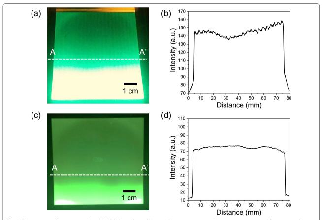
**Fig. 9** Emission test and intensity analysis of OLED lighting device (70 mm × 70 mm emission area); **a** an emission image and **b** an intensity line profile for the OLED lighting device fabricated with the PEDOT:PSS thin film coated by the micro single-nozzle jet head, **c** an emission image and **d** an intensity line profile for the OLED lighting device fabricated with the PEDOT:PSS thin film coated by the micro multi-nozzle jet head
