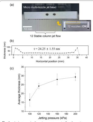
**Fig. 6 a** A photograph of continuous stream jet flow formation, **b** thickness profile of the single-path coated PEDOT:PSS pattern, **c** average thickness change of the single-path coated PEDOT:PSS films for the applied jetting pneumatic pressure of 100, 120, 160, and 200 kPa
