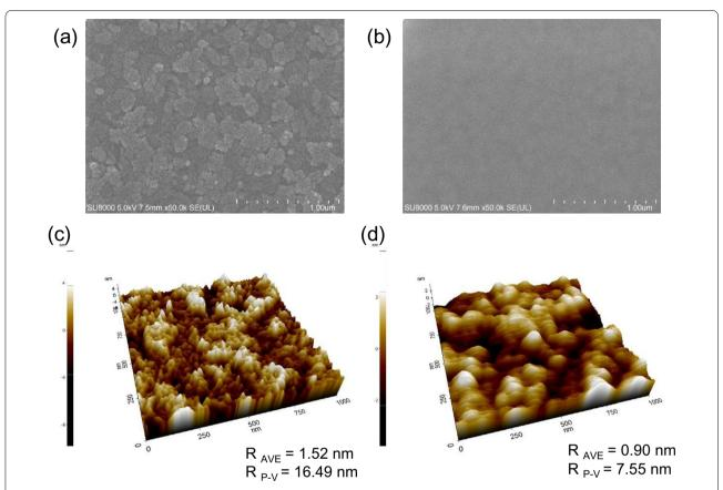
**Fig. 7** Surface topography analysis results: SEM images of **a** a bare ITO-deposited glass surface and **b** PEDOT:PSS film surface deposited on the ITO-deposited glass by micro multi-nozzle jet coating, **c** AFM images of **a** a bare ITO-coated glass and **d** PEDOT:PSS film surface deposited on the ITO-deposited glass by micro multi-nozzle jet coating
