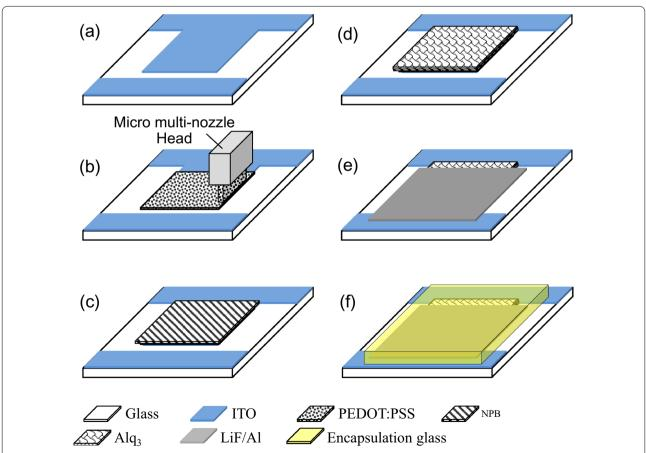
Fig. 2 The fabrication flow diagram of the OLED lighting device: **a** ITO electrode patterning, **b** PEDOT:PSS layer (HIL) coating using a micro multi-nozzle jet head, **c** NPB patterning, **d** Alq<sub>3</sub> patterning, **e** LiF/Al patterning, and **f** encapsulation
