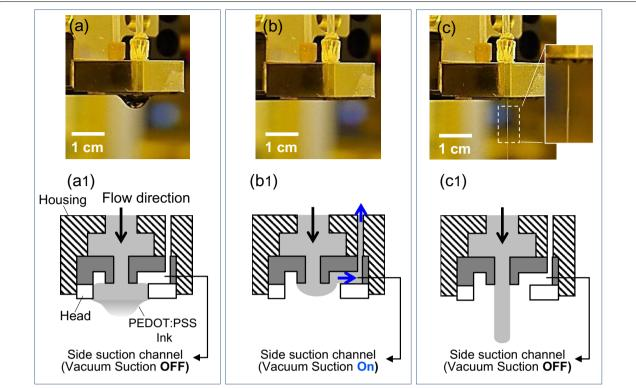
**Fig. 4** Sequential photographs of the micro single-nozzle jetting by applying vacuum suction to the side of the jetting nozzle: **a–c** photograph images around the tip of a nozzle, **a1–c1** cross-sectional schematic diagram of jetting (modified from Shin et al. [23, 24])
