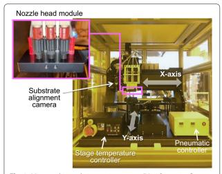
**Fig. 1** Micro multi-nozzle jet coating system (Mini Streamjet Coater, DEVICEENG, Korea). The inset image shows an enlarged nozzle head module photograph
