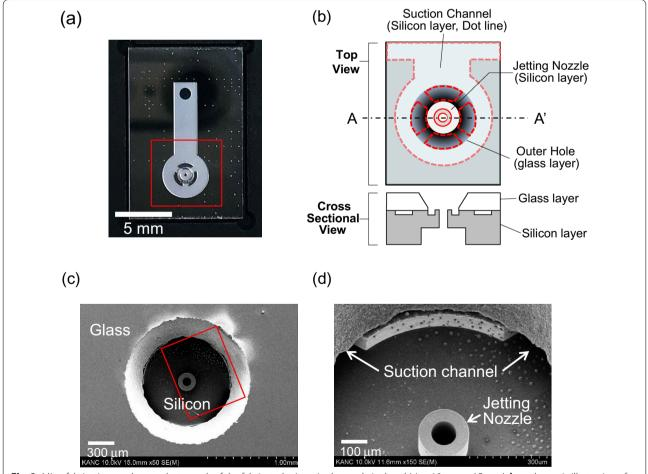
Fig. 3 Microfabrication results: **a** a photograph of the fabricated micro single-nozzle jet head (size: 10 mm × 15 mm), **b** a schematic illustration of part of a micro single-nozzle jet plate denoted by the red square in **a**, **c** SEM images of **c** a jetting nozzle part and **d** the enlarged jetting nozzle part indicated by the red square in **c**
