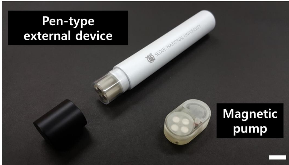
Figure 3.6 Optical image of the pump and external device with patterned magnets. The scale bar is 1 cm.
