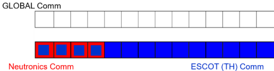
Fig. 4.2: coupling topology between the neutronics solver and the ESCOT code.
