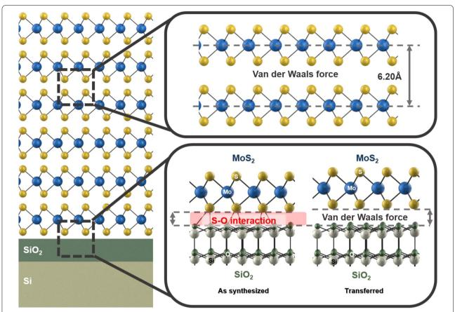
**Fig. 6** Schematic illustration of the phenomena at the AS and TR-MoS $_2$ /SiO $_2$  interface. At the AS-MoS $_2$ /SiO $_2$  interface, the interlayer distance decreases due to the formation of S–O bonding, whereas there is no significant change in the interlayer distance at the TR-MoS $_2$ /SiO $_2$  interface
