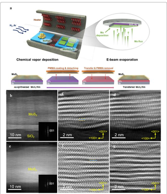
**Fig. 1** a Schematic illustration of the  $MoS_2$  film deposition and transfer. STEM images of  $MoS_2$  film on  $SiO_2$ /Si. **b** Low-magnification HAADF STEM, **c** Cs-corrected ABF STEM, and **d** Cs-corrected HAADF STEM images of AS- $MoS_2$  film. **e** Low-magnification HAADF STEM, **f** Cs-corrected ABF STEM, and **g** Cs-corrected HAADF STEM images of TR- $MoS_2$  film
