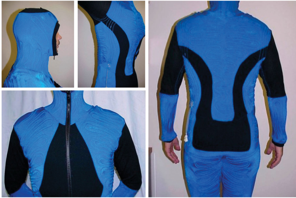
Figure 2. Subject wearing the liquid cooling garment (LCG) used in the study. Note: Several different views presented. The LCG is designed to cover areas of the body with high heat exchange capacity. The full color version of this figure is available online (National Institute for Occupational Safety and Health [NIOSH] file photograph).
