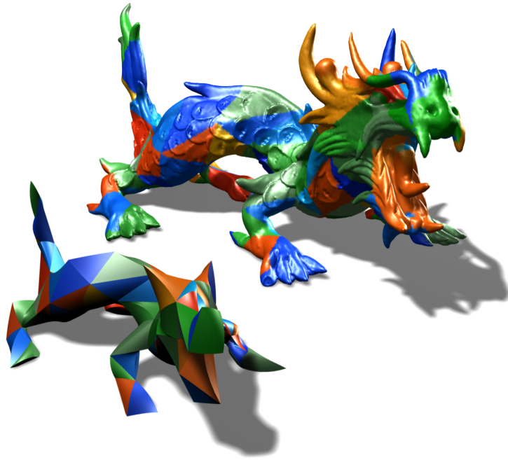
Figure 10. Dragon: 100.000 surface vertices, 173 quadratic tetrahedra. The surface colours visualise the mapping to the boundary tetrahedra.
