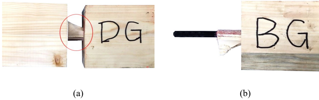
267 Fig. 5. Failure modes: (a) in timber joints with the glued-in DW dowels; and (b) in 268 timber joints with the glued-in threaded steel rods.
