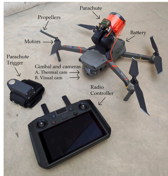
Fig. 7. Aerial measurement device – DJI Mavic 2 Enterprise Advanced.
