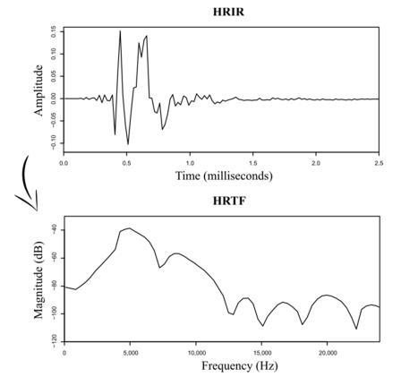
**Figure 2.** Relation between HRIR and HRTF. Example: 'A' pinna,  $\theta = 190^{\circ}$ ,  $\phi = -45^{\circ}$ .
