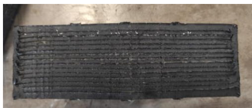
Figure 8 – Swelling of the under-vulcanized device.
