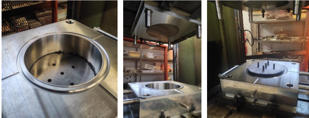
Figure 3: Steel mold for the UFREI fabrication
