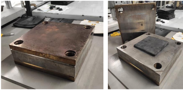
Figure 2: Steel mold for the UFREI fabrication
