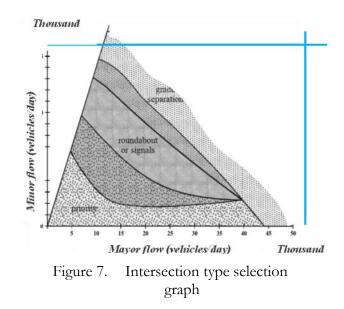
Based on the graph in figure 7 above, it can be concluded that the type of intersection that is suitable for the Kodim Intersection is a non-level intersection; therefore, an alternative solution will be made to change the geometric intersection to be symmetrical and make a flyover on the minor arm. So that the sketch of the intersection can be seen in figure 8.
