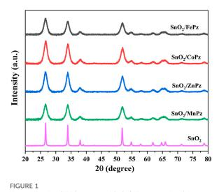
X-ray diffraction (XRD) patterns of SnO\_2/MPz composites (M = Fe^{2+}, Co^{2+}, Zn^{2+}, and Mn^{2+}).
