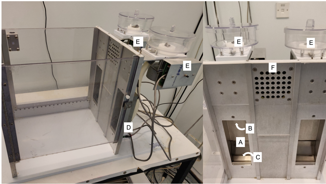
Figure 3.1: Annotated photograph of rat operant chamber. A side view (left) and front view (right) photograph of a representative operant chamber where rats performed the interval timing task, with operant chamber ports (A) equipped with stimulus light (B) and receptacle (C) with IR head entry detector (D). The left port is the “hold port” in which rats have to sustain nose poke fixation during a sound emitted through the speaker (F). The right port is connected to a pellet dispenser (E) and is thus used as the “reward port”.
