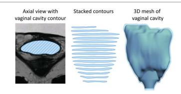
Figure 2. The anthropomorphic vaginal wall model was made using vaginal wall contours drawn in axial MR images. A generic cylindrical base was added to the model. Reproduced From [6]. CC BY 4.0.
