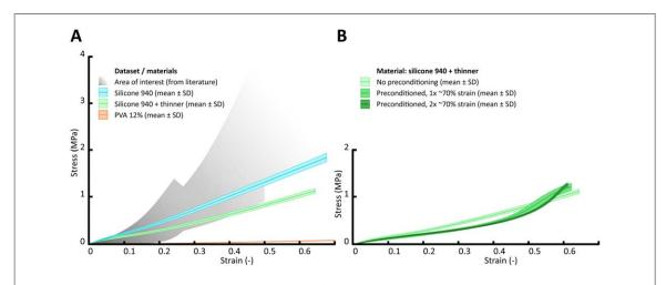
$\textbf{Figure 5.} Stress-strain curves obtained by uniaxial tensile tests of Silicone 940, Silicone 940+ thinner, and PVA 12\% dog-bone samples (A). The effect of material preconditioning is shown by applying 1–3 times a $\sim 70\%$ strain on the samples (B).}$
