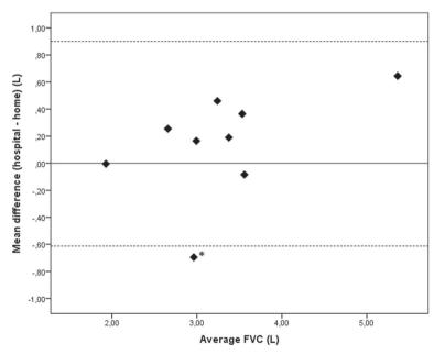
**Figure 2:** Bland-Altman plot comparing hospital and home spirometry. The value for hospital FVC is the mean of the hospital-based FVC at baseline and after four weeks. The value for home spirometry is the mean of 28 home FVC readings. The solid line represents the mean difference and the dashed lines 95% limits of agreement (-0.61 to 0.90L).\* This patient did not use the mouthpiece correctly leading to more variable and higher readings compared to hospital spirometry.
