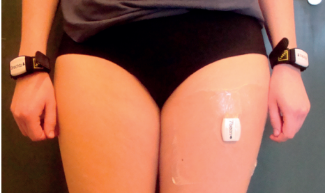
Figure 5.2 Placement of the three Activ8s of the Activ8-AUM device.
