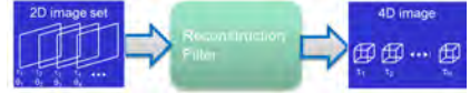
Figure 2.4: The 4D image reconstruction scheme. The input 2D image set with angle and cardiac phase information is fed into the reconstruction filter which creates a series of 3D time frames by using either normalized convolution (NC), nearest neighbor (NN) or linear interpolation with temporal binning (LTB).
