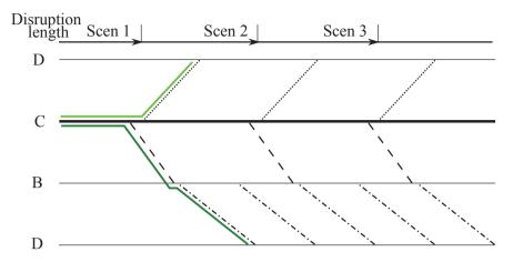
Figure 5.3: Time-space representation of the timetable between stations C and D. (Note that two time-lines are associated with station D in order to avoid crossing lines.)
