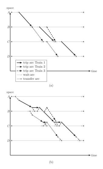
Figure 2.3: The Basic Network Formulation (a) and the Extended Network formulation (b) of a 4 station network with 3 different trains.
