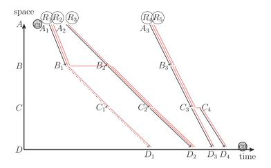
Figure 2.4: Time-Space diagram of five candidate routes for a journey with a check-in (ci) at station A and a check-out (co) at station D.
