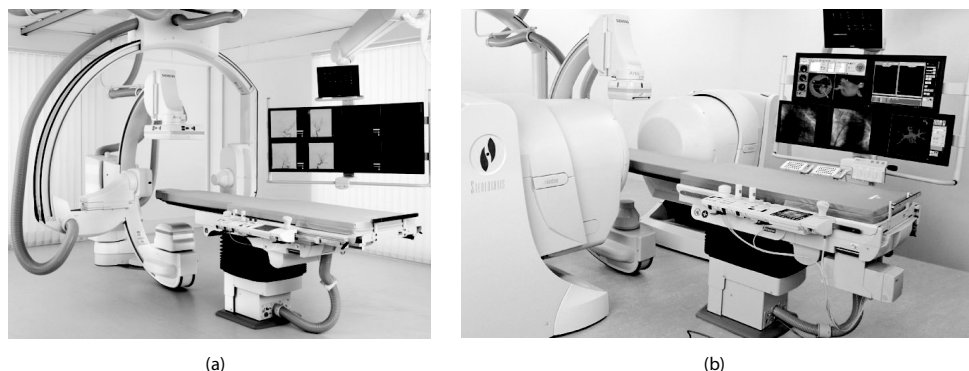
Figure 1.4: Typical set-up of (a) a normal angiography room, with a Siemens Artis zee biplane X-ray system and (b) a angiography room enabled for magnetic navigation. In (b) the two magnets left and right of the table generating the magnetic field are clearly visible (images copyright Siemens AG).
