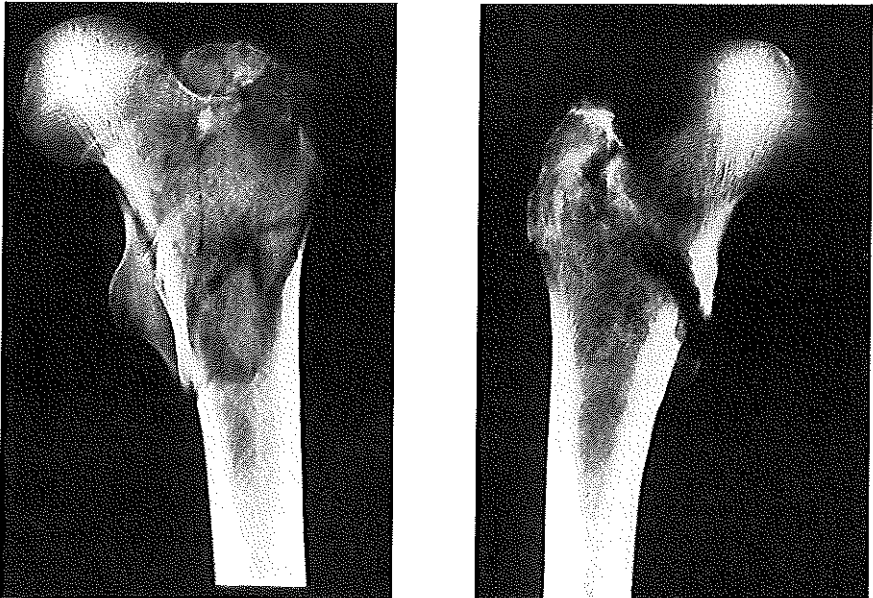
Figure 8.1 - Two radiographs of fractures after mechanical testing
