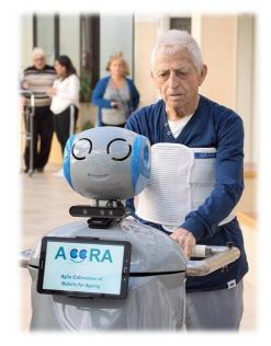
Astro is a robot for mobility assistance and rehabilitation, used in hospitals or retirement homes. This robot was developed by Santa Anna University in Italy.
