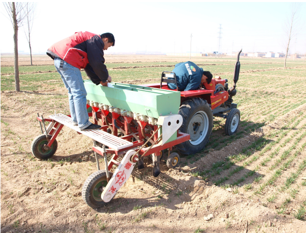
Picture 1: Modified seeding application attached to a small tractor typical for the NCP. These applications and tractors are widely used by local farmers.
