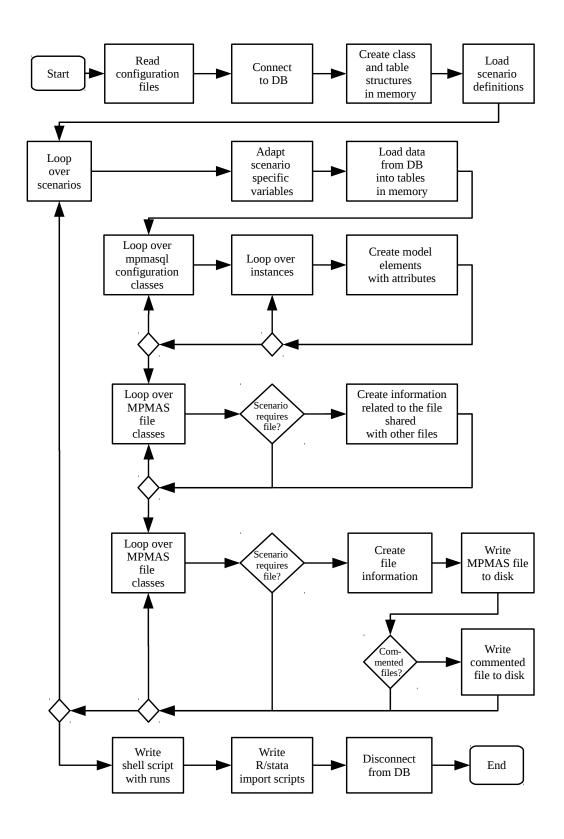
Figure 5.2: Flowchart of the MPMAS file creation process performed by mpmasql.
