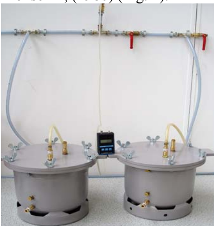
Fig. 2 Porosity apparatus adapted according Mohsenin, 1980
