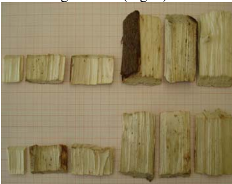
Fig. 1 Spruce wood chip groups used for air flow resistance determination.
