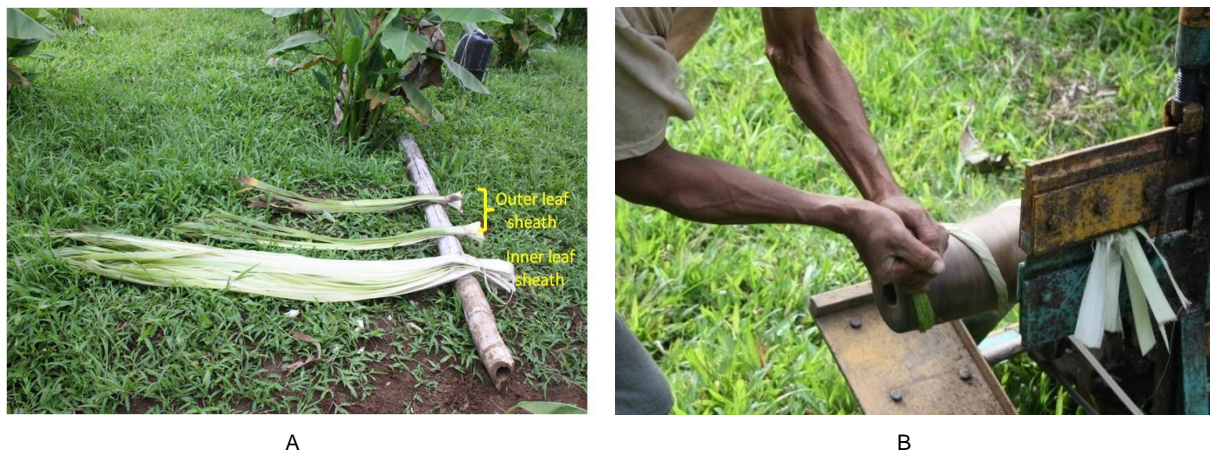
Photo 5.4 Tuxies from outer and inner leaf sheaths (A) and winding of tuxies (from the outer leaf sheaths) around the spindle of the stripping machine (B)
