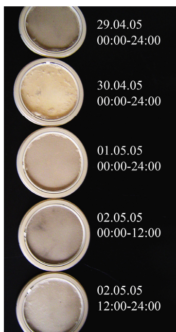
Figure 4.10: Loaded filters covering the period from 29 th of April to 2 nd of May 2005. Wind flows from south east leading air masses from south of Beijing city to DBW as shown by dark grey coloured filter on 29 th of April. Wind flows from north west leading air masses from desert regions to DBW as shown by yellow coloured filter on 30 th of April.
