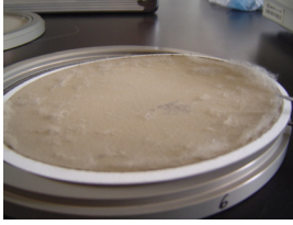
Figure 3.4: Overloaded filter with PM during dust storm event on 30 th April 2005.
