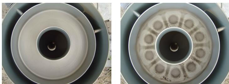
Figure 3.3: Top view on opened PM impactor before (right) and after (left) cleaning of impactor plate. Picture of dirty impactor was made after 5 days in operation. (all photos taken in 2006).
