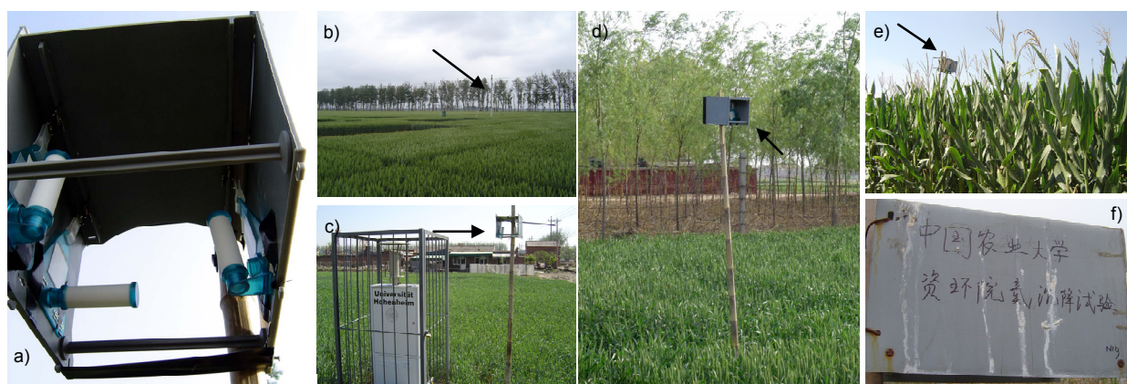
Figure 3.5: Passive sampler in operation: a) interior view of shelter with three replicates; b) at WU, winter wheat, arrow marks energy mast located in agricultural field where samplers were installed; c) at DBW, winter wheat, close to the High Volume Sampler; d) at QZ, winter wheat; e) at DWB, bamboo stick with samplers located in summer maize field; f) at DBW, contamination of shelter by birds (all photos taken in 2005).
