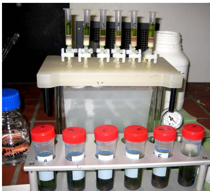
Fig. 5.2. SAX cartridges used for cleanup which leads to 20-fold enrichment, in order to improve the sensitivity for fumonisin detection.
