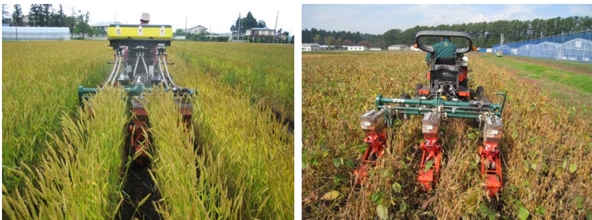
Fig. 14. Mechanized sowing of soybean into wheat (left) and wheat into soybean (right) in northern Japan using the “interseeder”. (Photos: Kouchi Amaha)
