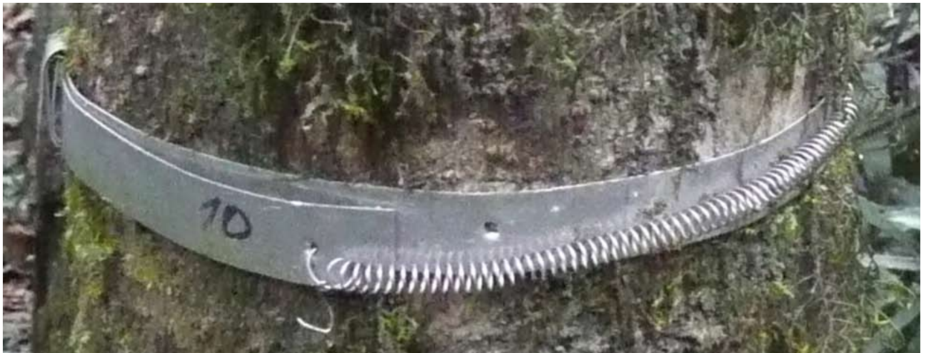
Figure 3-2: Example of a dendrometer mounted on a tree.
